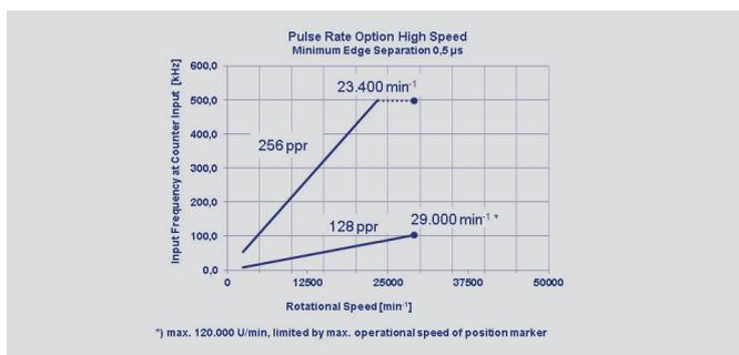
\*) max. 120.000 U/min, limited by max. operational speed of position marker
