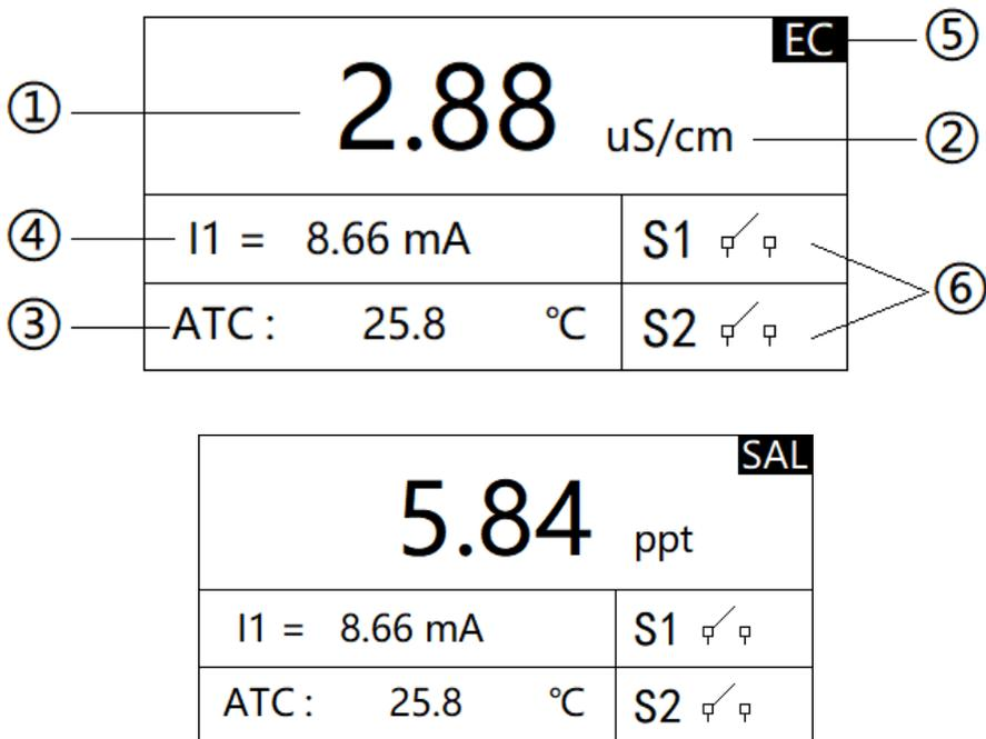
Figure 2 The main interface of measurement display
